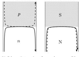
FIG. 24 Schematic top view of a graphene nanoribbon containing an interface between a p-doped and n-doped region (left panel) and between a normal (N) and superconducting (S) region (right panel). Electron-like and hole-like edge states in the lowest Landau level are indicated by solid and dashed lines, respectively, with arrows pointing in the direction of propagation. (Tworzydło et al., 2007)
